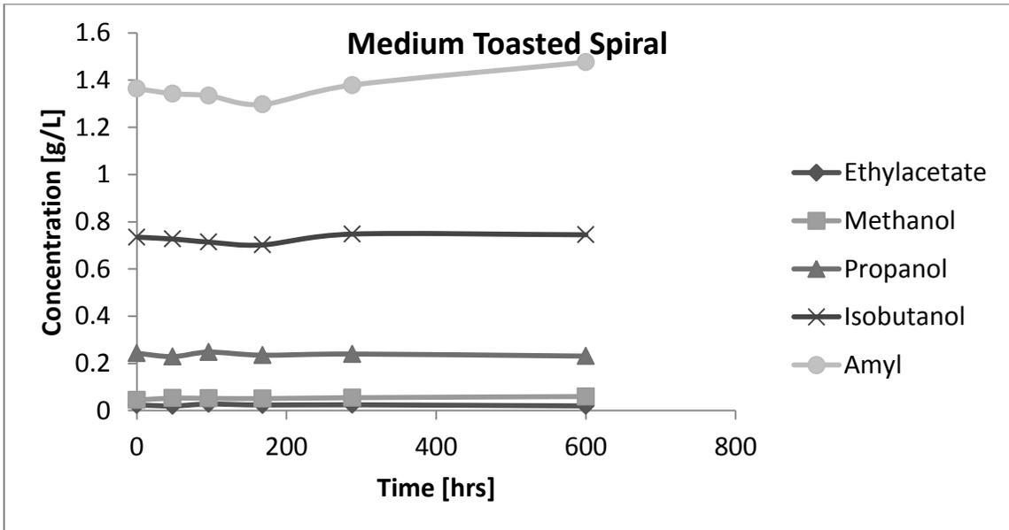
Figure 37: Volatile congener concentrations in Pyrex containers during exposure to medium toasted spiral over 25 days
