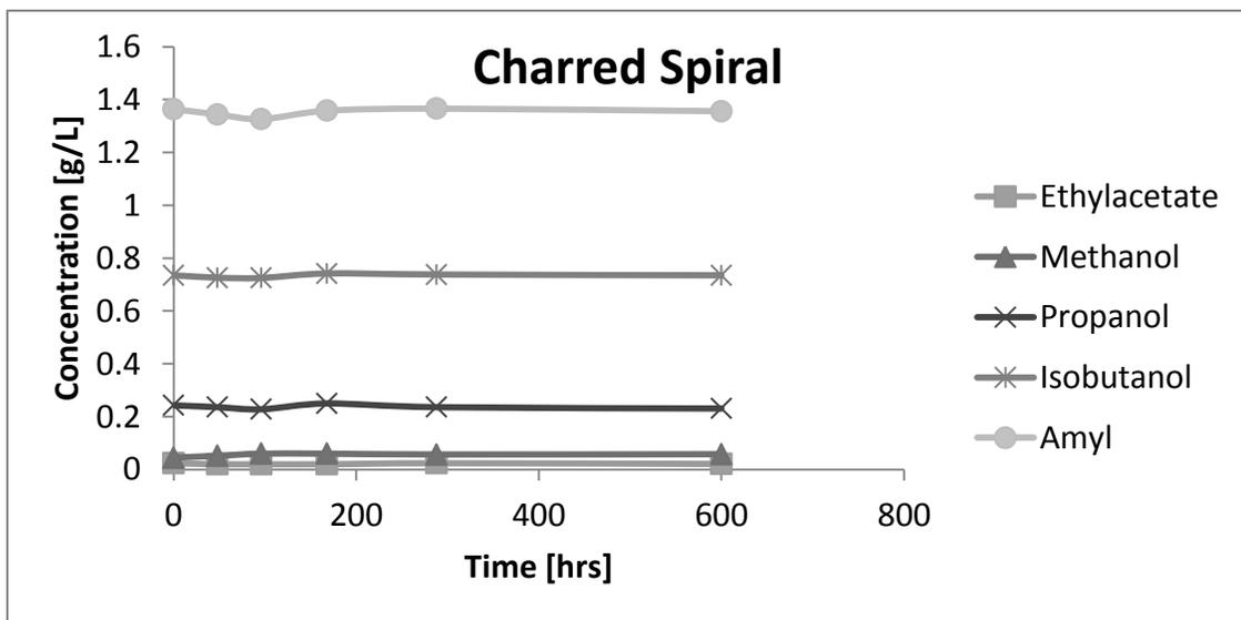
Figure 39: Volatile congener concentrations in Pyrex containers during exposure to charred spiral over 25 days
