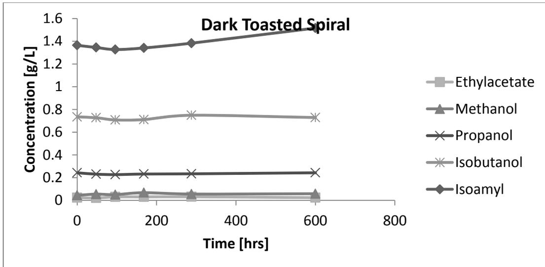
Figure 38: Volatile congener concentrations in Pyrex containers during exposure to dark toasted spiral over 25 days
