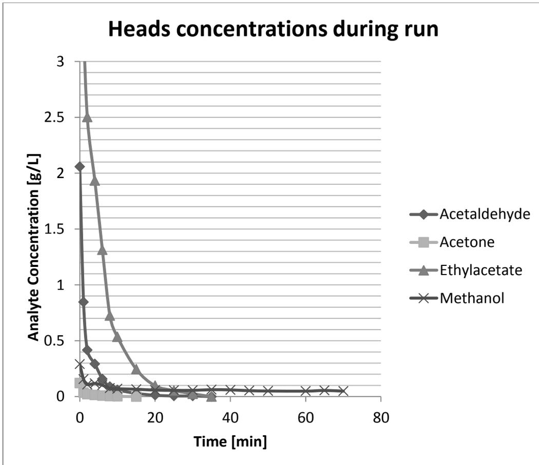
Figure 3: Showing the concentration of heads compounds over time in the distillation of a bourbon whiskey.
