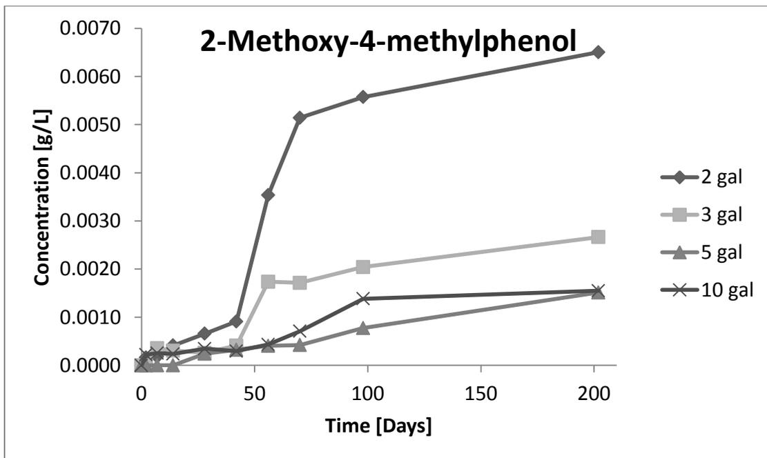
Figure 16: Averaged duplicate concentrations of 2-Methoxy-4-methylphenol over 202 days in all barrels
