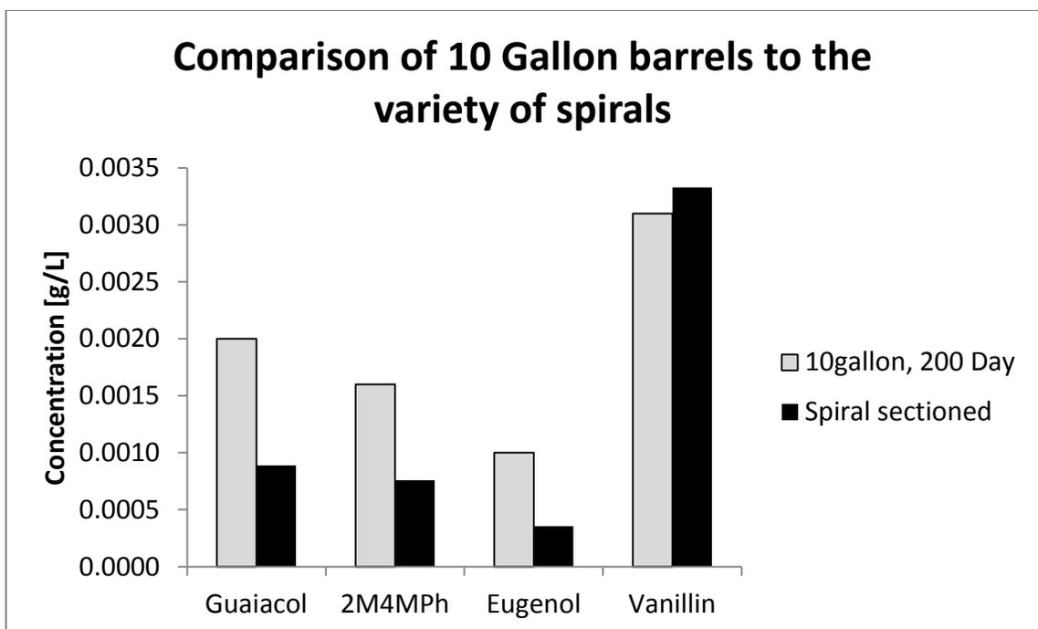
Figure 26: Concentrations of 4 compounds extracted from oak spirals combined and corrected for manufacturer recommended treatment, compared to those extracted from 10 gallon barrels
