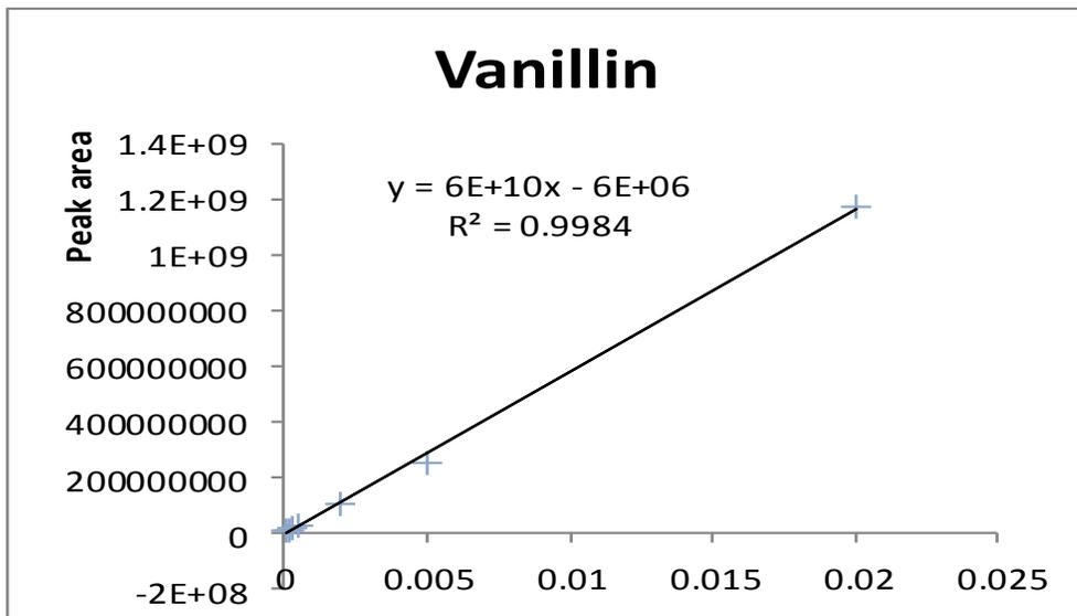
Figure 34: GCMS standard curve for vanillin concentration
