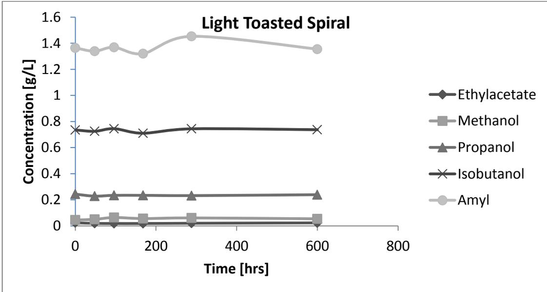
Figure 36: Volatile congener concentrations in Pyrex containers during exposure to light toasted oak spiral over 25 days
