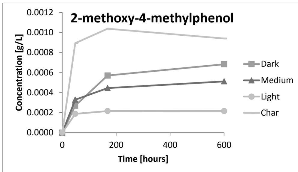
Figure 21: Concentrations of 2-methoxy-4-methylphenol extracted from oak spirals by whiskey spirit, over 600 hours (25 days)
