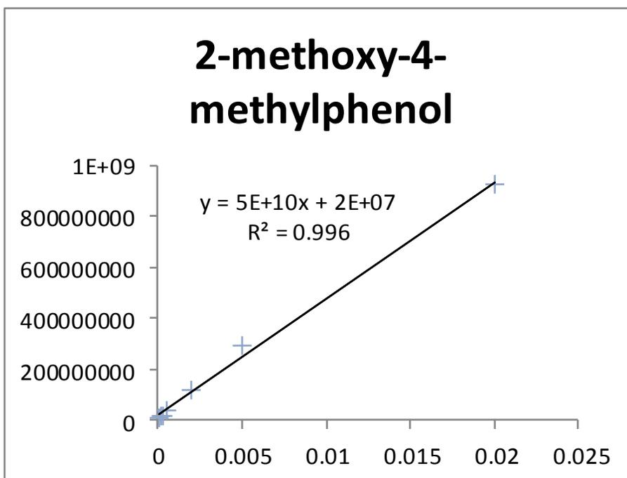
Figure 35: GCMS standard curve for 2-methoxy-4-methylphenol
