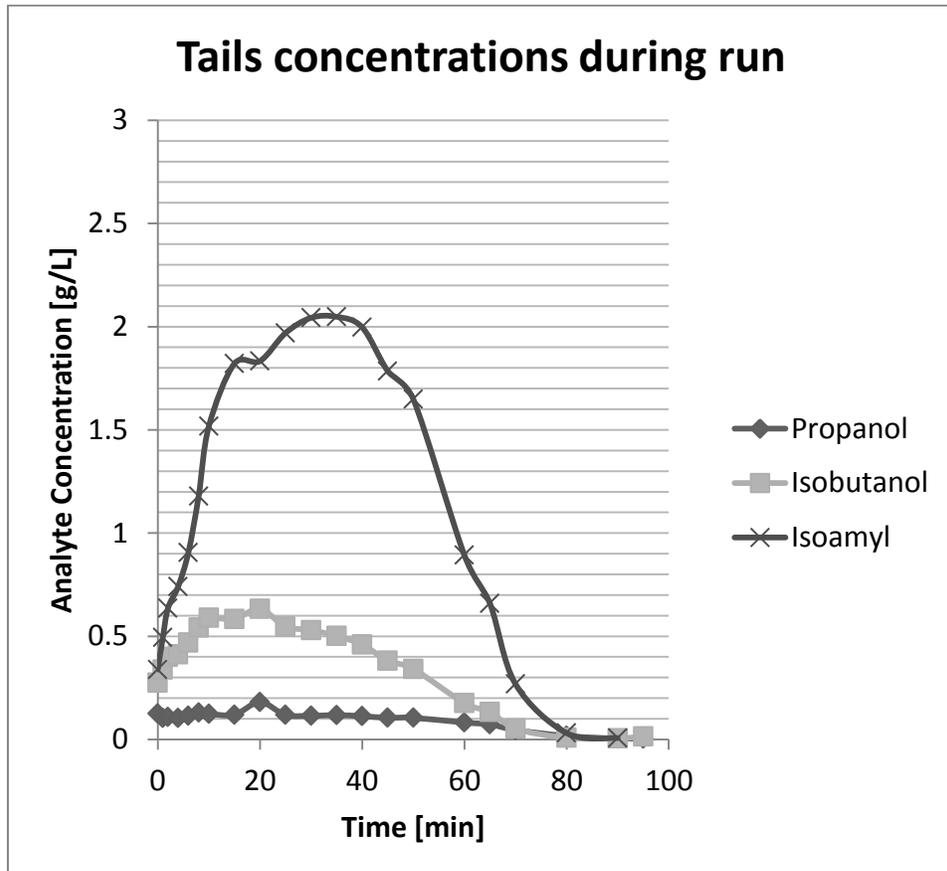
Figure 4: Showing the concentration of common higher alcohols during the distillation of a bourbon whiskey.
